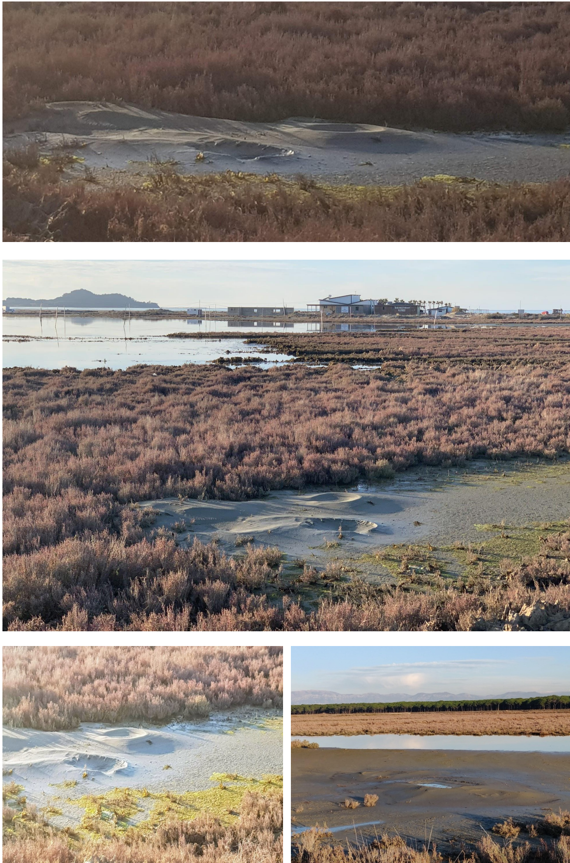
Figure 48: Sand boils and craters due to soil liquefaction in the bay of Porto Romano.
