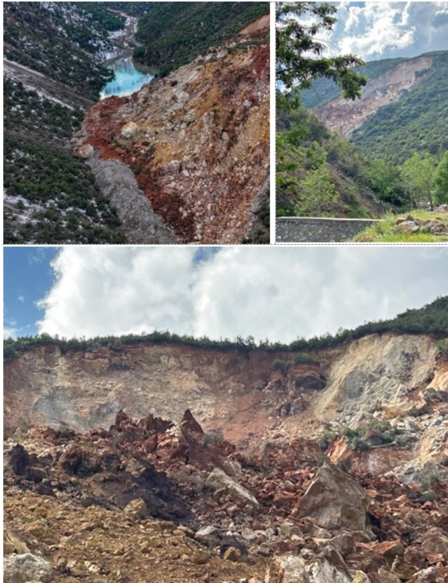
Figure 3.49 The rock mass is highly karstified and brecciated with high presence of clayey infilling material around rock fragments and along certain fractured sub-vertical zones.
