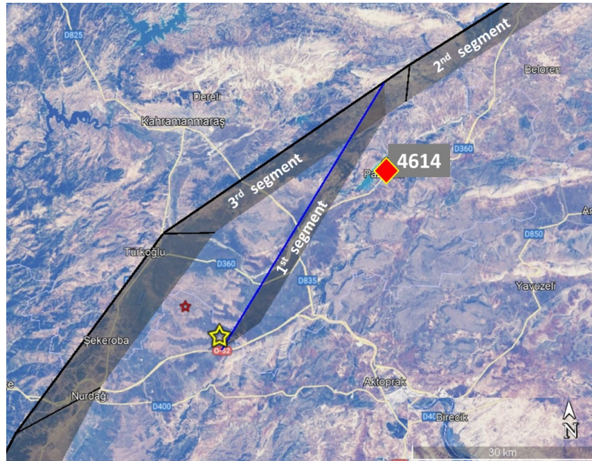
Figure 2.5 Map of the rupturing fault segments during Mw7.8 Pazarcik earthquake along with the location of station 4614 in which the greatest PGAs were recorded.
