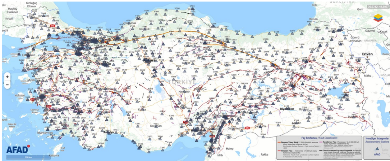
Figure 2.1 Map of the AFAD strong motion Network. The recording stations are shown with blue triangles.
