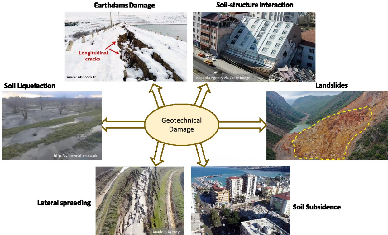
Figure 3.21 Geotechnical failure types observed in the 2023 Kahramanmaraş earthquake sequence.
