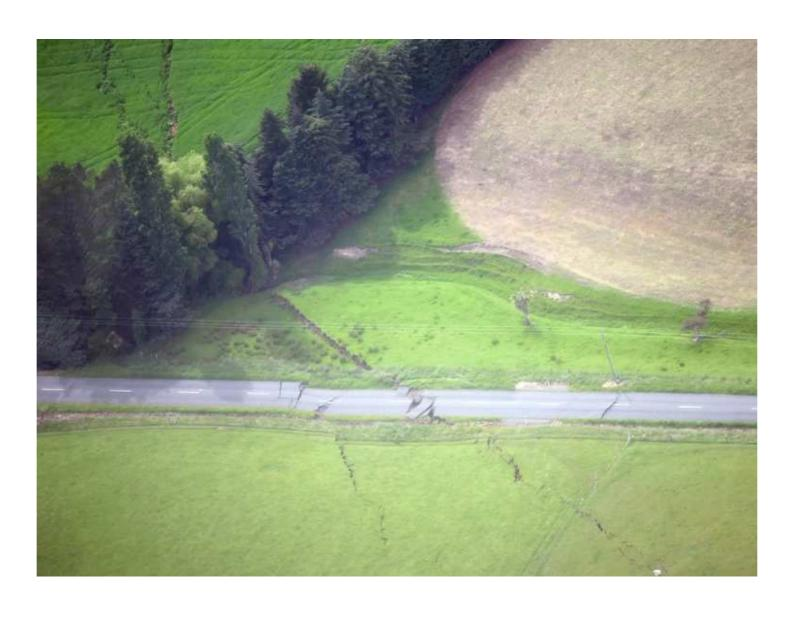
Right-Lateral Strike-Slip Fault rupture of the ground surface (\*near Kaikoura)
