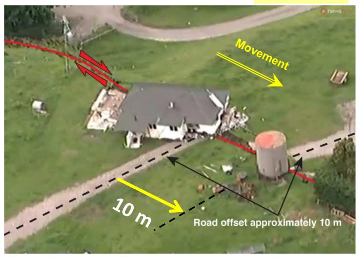
House moved and heavily damaged, but the cylindrical barn (or tank?) seems to have escaped damage (perhaps by fault "diversion"??)
